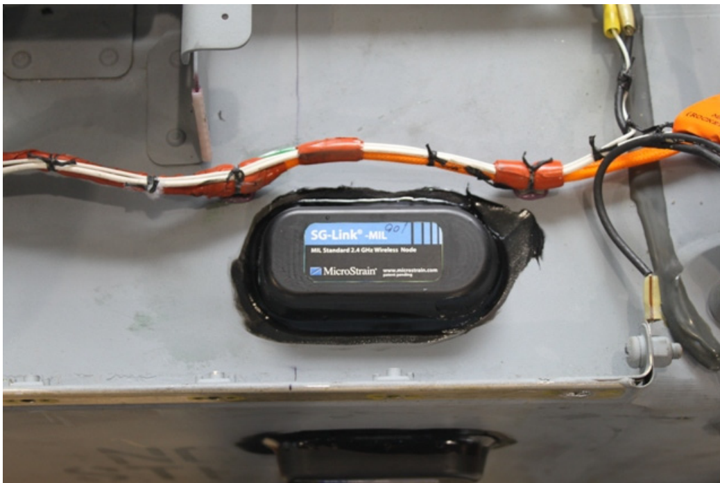
Figure 4: Wireless strain sensor node (SG-Link-MIL) installed aboard MH-60S
