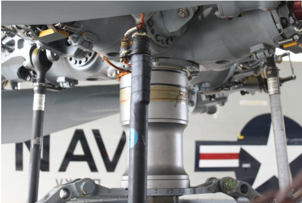
Figure 4: Wireless strain sensor node (SG-Link-MIL) installed aboard MH-60S
