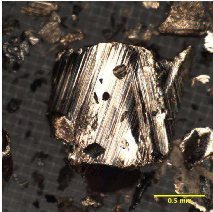
*Figure 2: Example of adhesive wear debris from morphology library showing characteristic striations across the surface*
