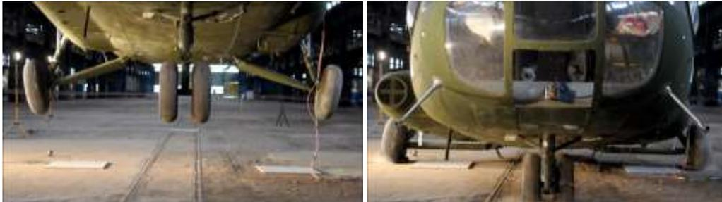
Figure 5 – helicopter before release and at maximum strut compression
