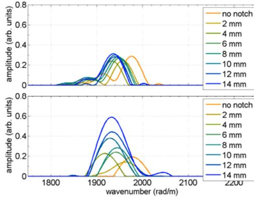
Fig. 4: Wavenumber profile at peak energy of the mode converted  $S_0$  mode downstream of the notch (bottom) as its length is increased. The wavenumber profile upstream of the notch is shown (top) for reference.
