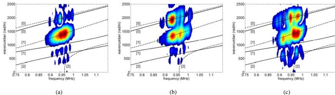
Fig. 7: Spectral decomposition based on a low spatial resolution of the wave field at 950 kHz for (a) pristine plate; (b) a 14 mm long, 1 mm deep notch and (c) a 14 mm long, 2.5 mm deep notch.
