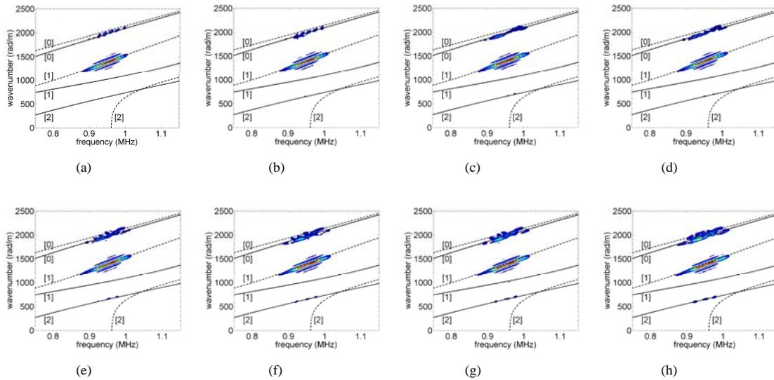
Fig. 3: Downstream spectral decomposition for (a) no notch; (b) 2 mm; (c) 4 mm; (d) 6 mm; (e) 8 mm; (f) 10 mm; (g) 12 mm; (h) 14 mm long notch.
