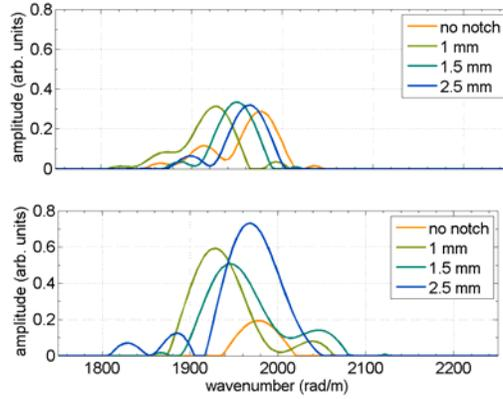
Fig. 6: Wavenumber profile at peak energy of the mode converted  $S_0$  mode downstream of the notch (bottom) as the depth is increased. The wavenumber profile upstream of the notch is shown (top) for reference.
