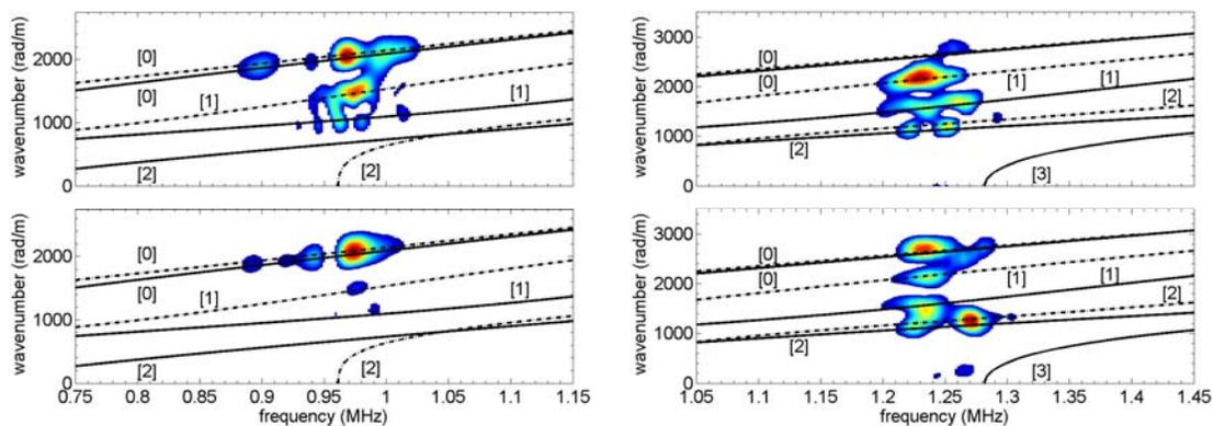
Fig. 8: Spectral decomposition of wave field acquired using FBG sensor array at 950 kHz (left) and 1.25 MHz (right). The top figures show the results for the plate in pristine condition and the bottom figures for the plate with a notch.
