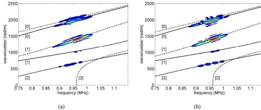
Fig. 5: Downstream spectral decomposition for (a) 1.5 mm; (b) 2.5 mm deep notch.
