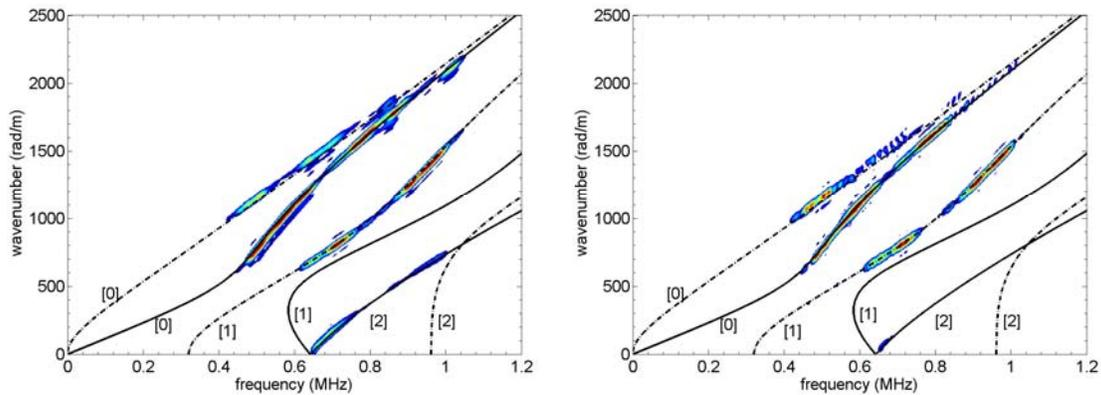
Fig. 2: Upstream (left) and downstream (right) spectral decomposition for pristine plate. Dotted lines denote dispersions lines for antisymmetric modes and solid lines for symmetric modes. The modal order is given in parentheses.
