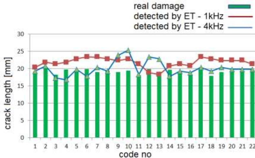
Fig. 11 Comparison of the actual crack length with operator measurements after patch application
