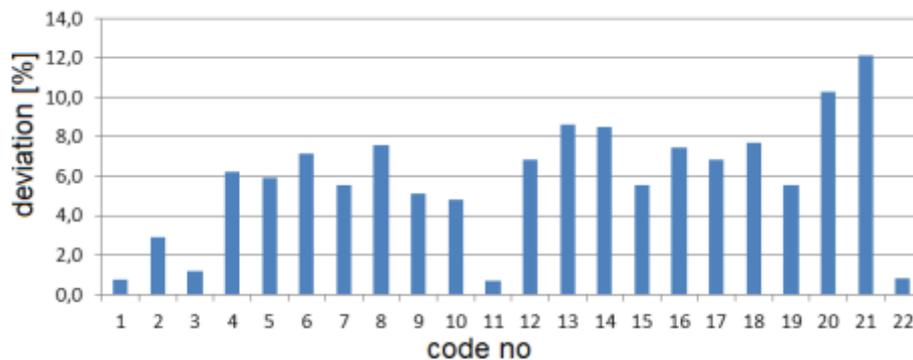
Fig. 12 Deviation of the crack length measurement, ET method
