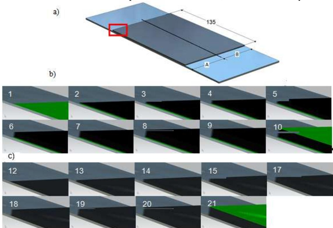
Fig. 3 Test article schematics, including article code number: a) patch dimensions A-patch applied, B- patch debondings, b) CFRP patch samples and layer count (layer thickness 0,15mm), b) CFRP patch samples and layer count (layer thickness 0,15mm)
