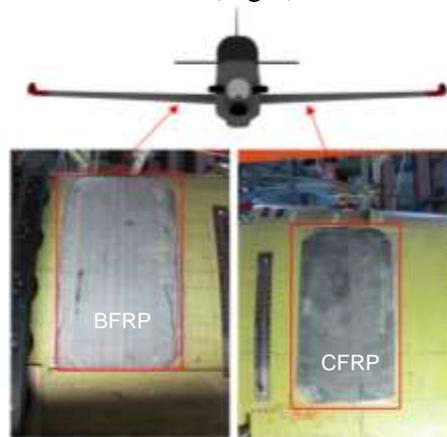
Fig. 1 *Location of composite repair patches on the PZL-130 Orlik TC-II aircraft test article*
