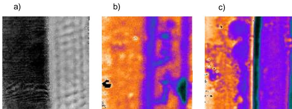
Fig. 9 Example inspection results (coupon no 5): a) MIA -18kHz, b) RT-170kHz, c) RT-270kHz
