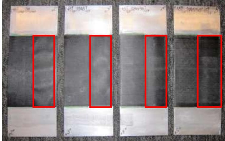
Fig. 4 coupon examples; red are is the debonding region
