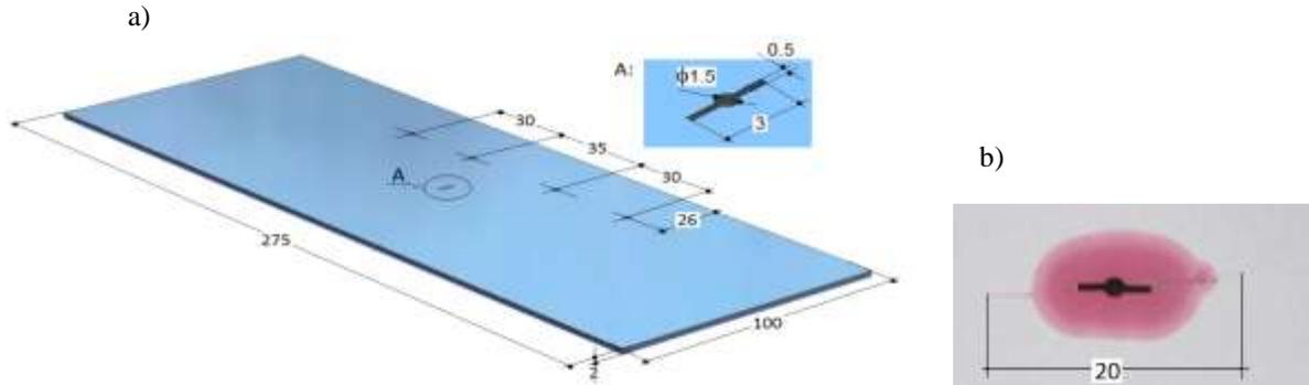
Fig. 2 Comparative coupon without patch: a) schematics – defect dimensions, b) view of actual modelled damage article code no 22
