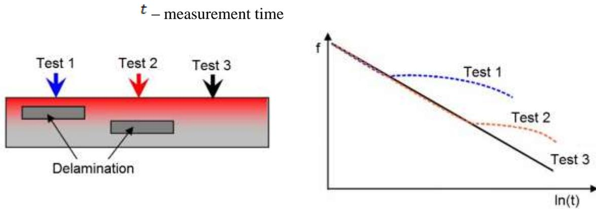
Fig. 6 Defect detection with the use of impulse thermography
