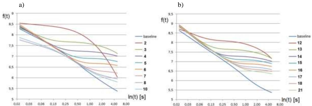
Fig. 7 Cooling curves: a) CFRP patch coupons, b) BFRP patch coupons
