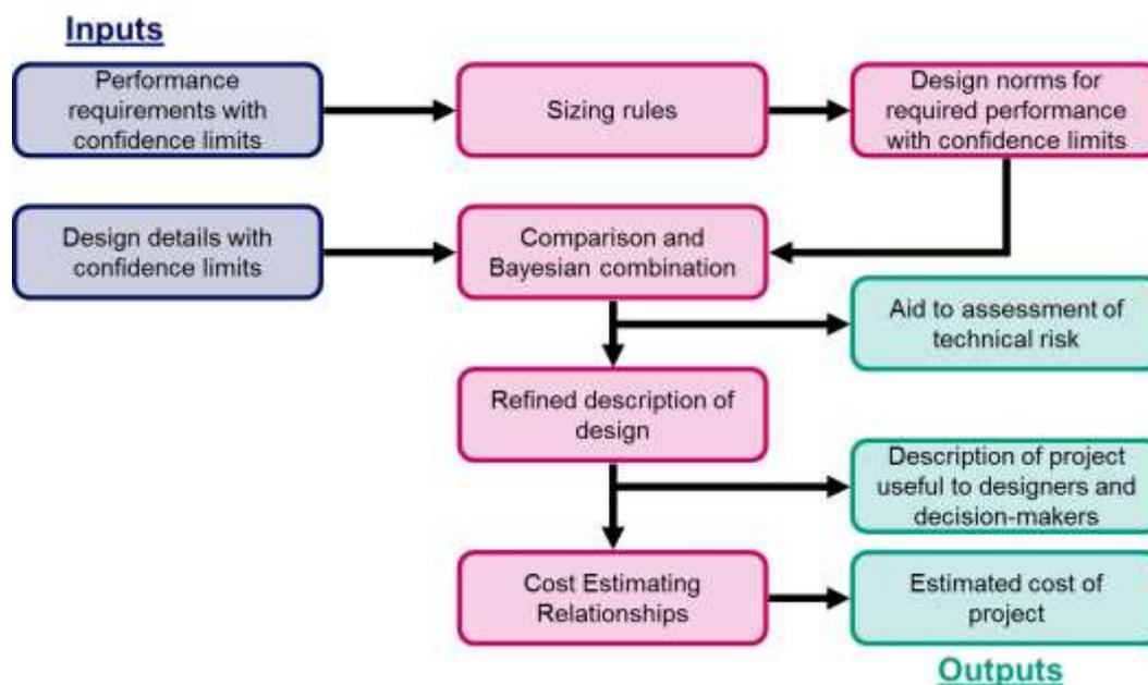
Figure 5: FACET estimating process with the application of Bayesian
