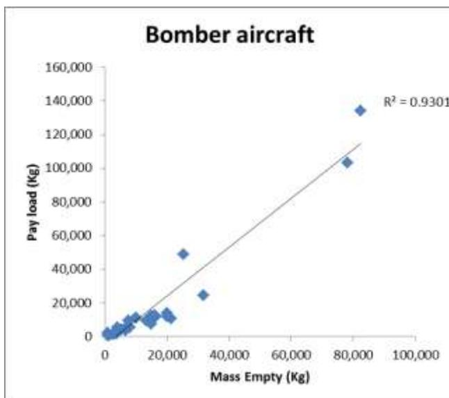
Figure 4: bomber aircraft design and performance characteristics exhibiting correlation
