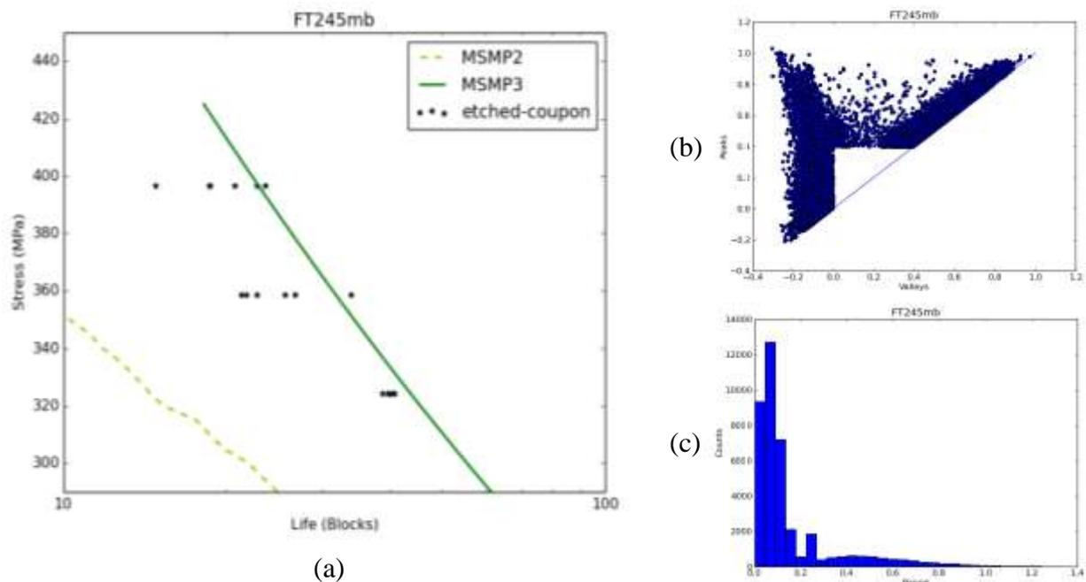
Fig. 4: (a) Comparison of predictions against etched coupon test lives for the wing test sequence FT245mb which contains numerous small buffet loads (b) peak-valley distribution of the cycles in the FT245mb sequence (c) histogram of the cycle ranges of the sequence. MSMP3 does a better job in correctly estimating the coupon lives than the MSMP2-relative version which is currently used to life aircraft
