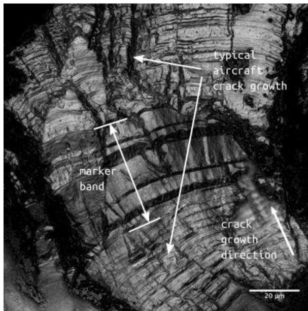
*Fig. 3: Marker band sequence inserted into typical blocks of spectrum loading. This technique has been used to measure the rate of crack growth in typical blocks of F/A-18 wing root bending moment loading*
