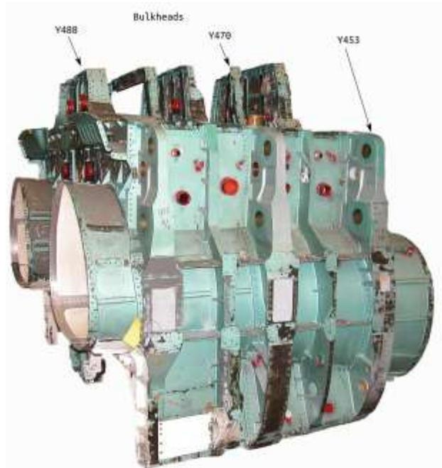
*Fig. 1: Centre-barrel of the F/A-18 A/B Hornet*
