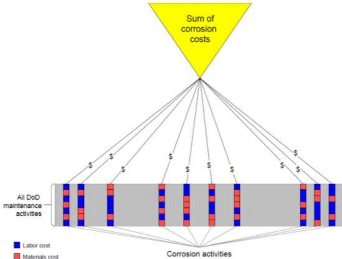
*Fig.2: Bottom-Up Corrosion Cost Measurement Method [11]*
