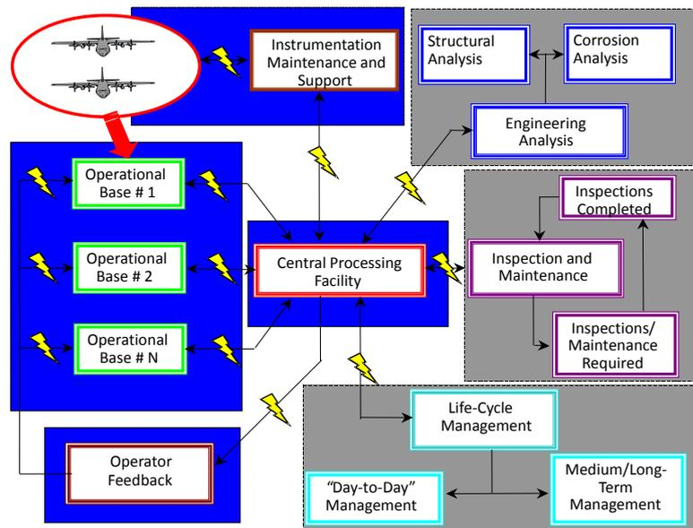
Figure 3: Overview of Typical Fleet Data Acquisition Process
