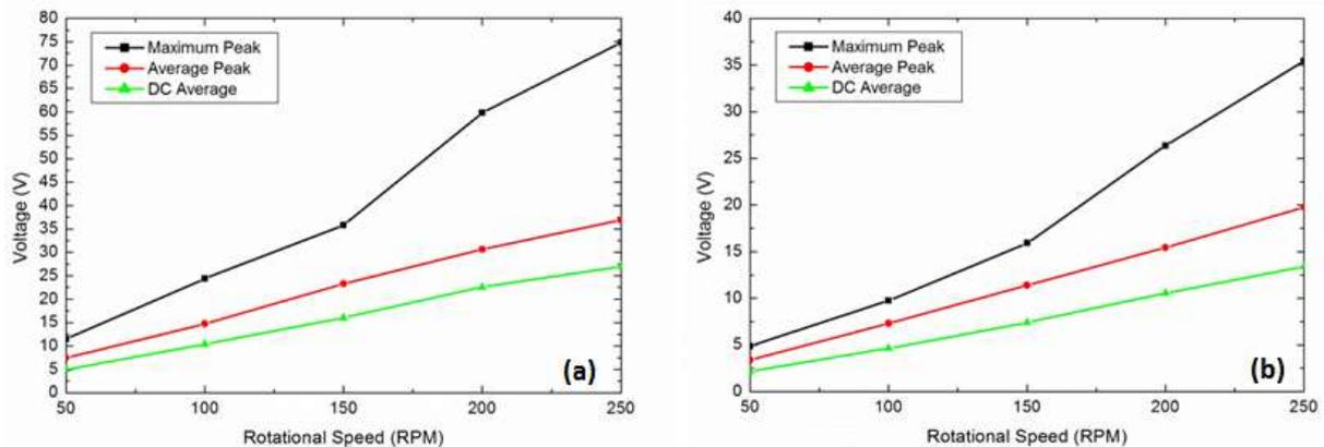
Fig. 5: a) Measured open circuit voltage, and b) measured load voltage across a  $750\Omega$  load, versus rotational speed.
