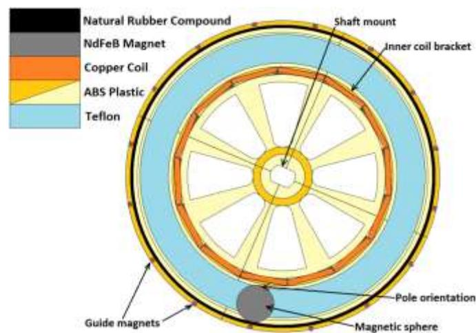
*Fig. 1: Showing the prototype rotational energy harvester wheel with key components labelled and materials highlighted.*
