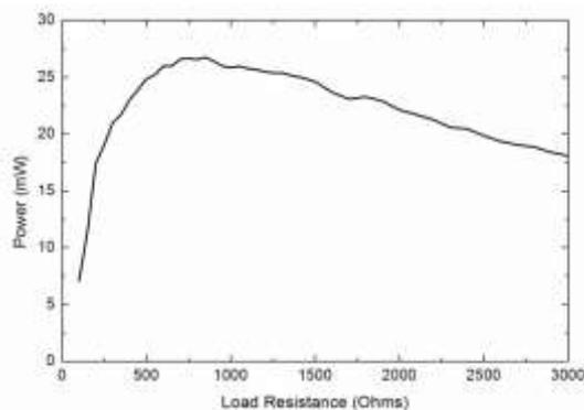
*Fig. 4: Measured average power versus load resistance.*
