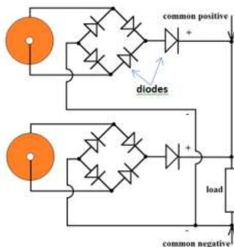
*Fig. 2: Showing wiring for two of the fourteen coils. Other coils are connected to the same load at the same common nodes.*
