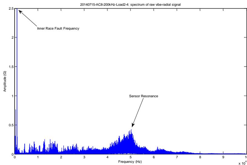
Figure 4. Spectrum of raw vibration signal shown in Figure 3
