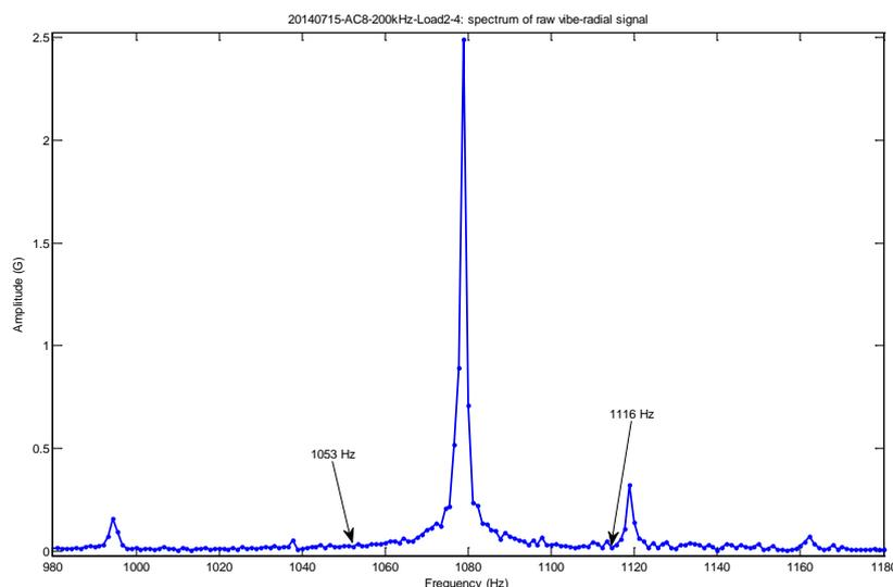
Figure 5. Identification of dominant bearing fault frequency in the spectrum of raw vibration signal
