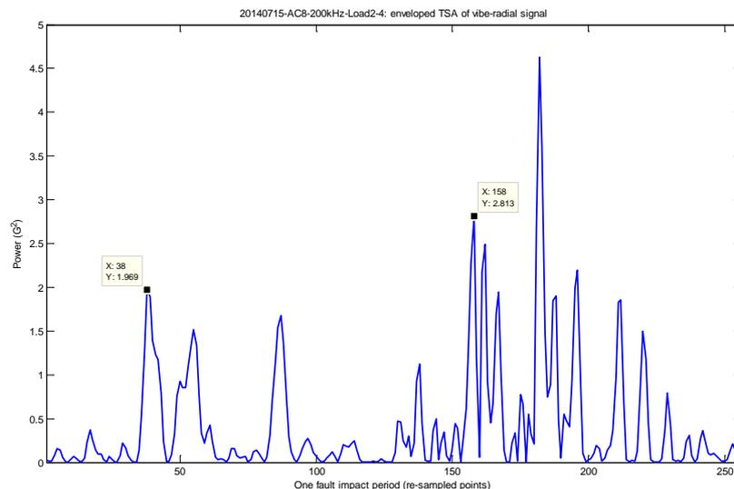
Figure 7. Enveloped TSA of AC8 (spall size estimate 4.7 mm)
