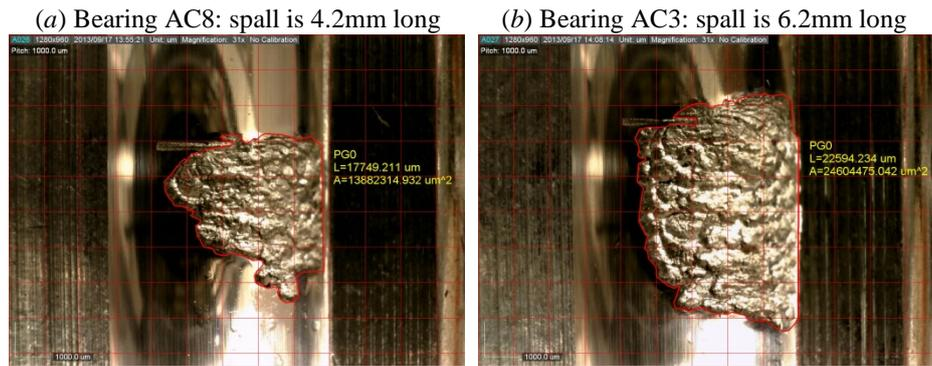
Figure 2. Pictures of the spalls on the inner race of Bearings AC8 & AC3
