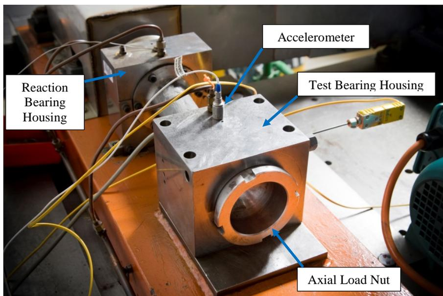
*Figure 1. DSTO Bearing test rig*
