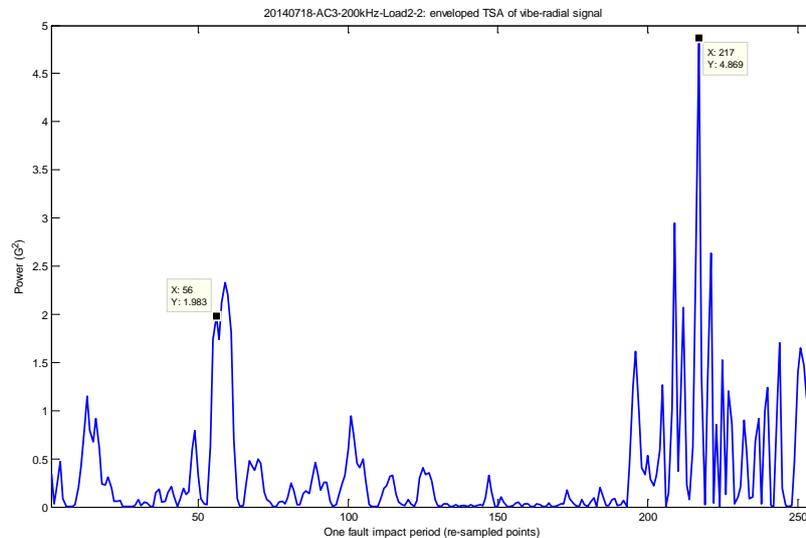
Figure 8. Enveloped TSA of AC3 (spall size estimate 5.9 mm)
