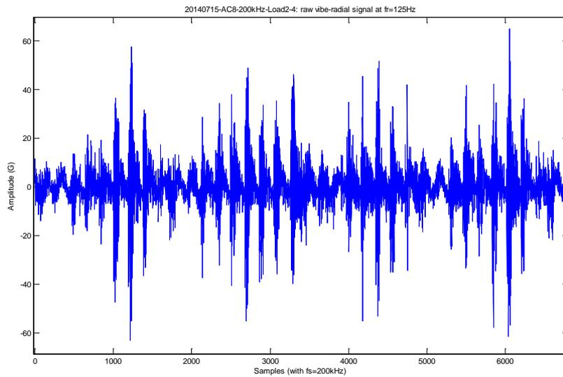
Figure 3. Raw vibration signal with Bearing AC8
