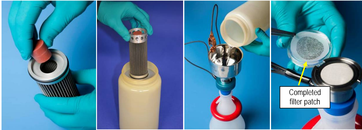
Fig.6: Manual filter debris extraction process using filter patch method
