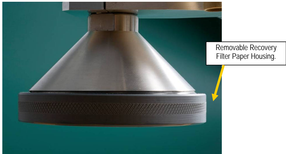
Fig.4: Recovery Stage showing divergant shape and removable recovery filter paper housing
