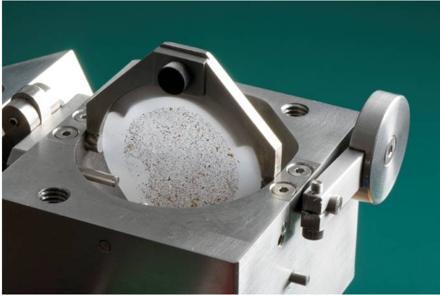
Fig.8: Entry Stage showing filter patch in the rotated position
