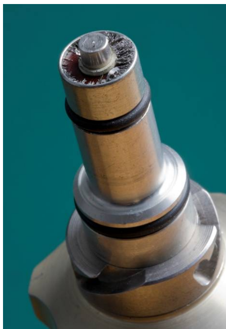
Fig.10: Common magnetic chip detector with debris
