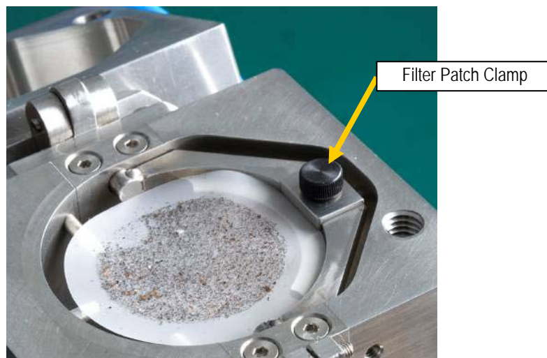
Fig. 7: Entry Stage showing filter patch clamped in installation position
