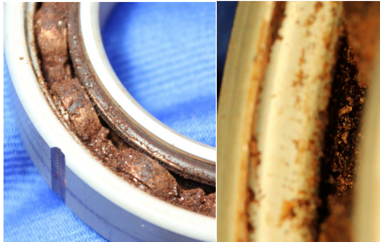
Figure 12 – Photographs of failed test bearing #4, (left) showing cage areas and (right) showing outer race surface between rolling elements
