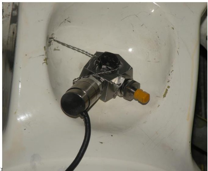
Figure 1: Sensor assembly installation on landing gear.
