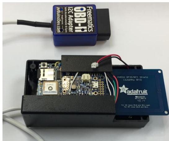
Fig. 3: Our custom-built OBD-II data logger, pictured with Freematics OBD-II Adapter
