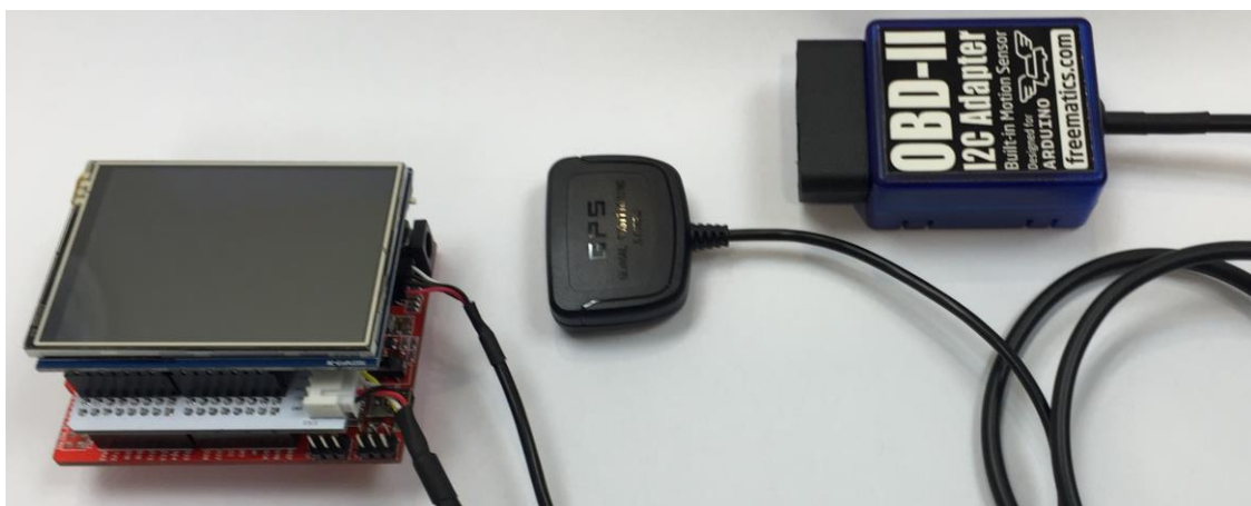
Fig. 2: Assembled Freematics OBD-II Telematics Kit #2, including external GPS receiver
