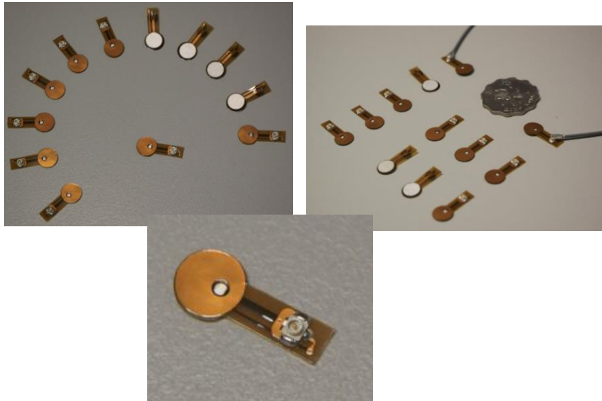
Decentralized sensing unit
