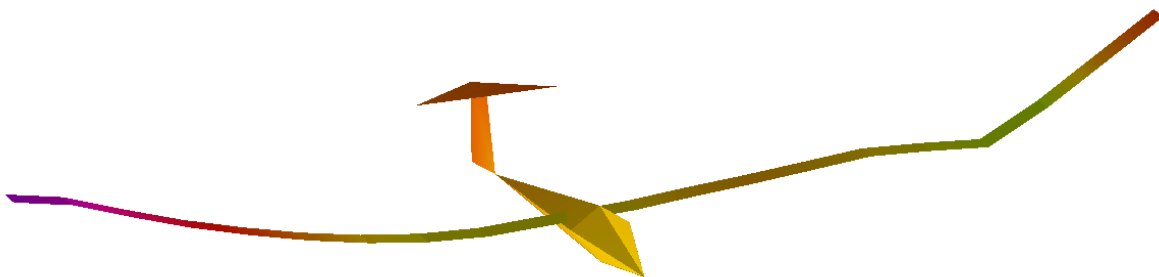
Fig. 6: S-WI-BX-1 Mode at 2.79 Hz from OMA 1
